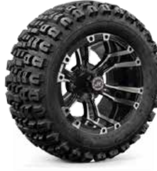
SET 240B1 23 x 10.50-12 K502 4PR TL Kenda Off Road 12 x 8 (-43 mm offset) 2RM240 + 2TR122 - $472
