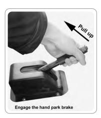
To disengage the parking brake, pull up the hand brake lever to the end and then press down the button on the top of the brake lever, with the button being pressed down, push down the brake lever to the bottom.
