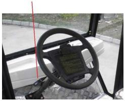
**Power key:** Controls the power supply of the whole vehicle. When the key is inserted into it and turned clockwise, it will switch on the lights, horn, and the control system; when the key is turned back, the power will be switched off.
