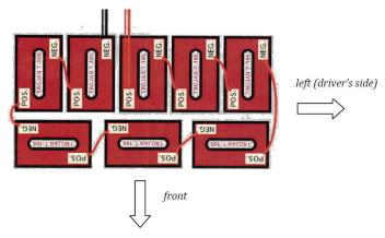
making sure that cables do not lay across vent caps. Always remove the negative (-) cable to the motor controller first, and install it last.
