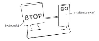
**Accelerator Pedal:** The accelerator pedal can be found on the right side labeled GO. This pedal is different from the accelerator pedal in common car. Turn on the main switch and select the F/R switch to move forward or in reverse and the golf car's speed will accelerate gradually as the accelerator pedal is depressed. Releasing the pedal causes the power to be cut and the motor to stop working gradually.
