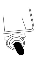
**Tow Switch:** The Tow switch is located in the front of the battery container. The switch can be seen clearly when the seat bottom is being opened by means of pulling the armrest forward. Pulling the switch to TOW (or OFF) will cut the power off and make the car stop.
