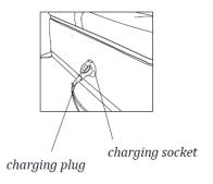
2. With the charger properly connected and grounded (see charger's owner's manual), insert the DC output plug into the golf car receptacle. Do not connect the AC with the golf car directly. CAUTION: Use only battery chargers that are rated for use with 48-volt Star EV Golf Cars. Thoroughly read and understand the user manual supplied with your 48-volt charger. WARNING: Do not disconnect the DC output cord from the
