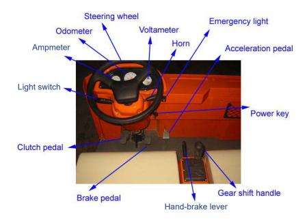
*Power key:* Controls the power supply of the whole vehicle. When the key is inserted into it and turned clockwise, it will switch on the lights, horn, and the control system; when the key is turned back, the power will be switched off.
