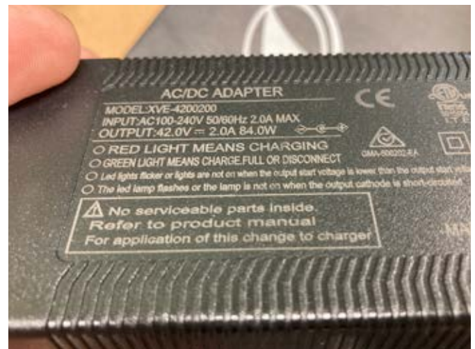
Lithium-internal/external pack charger specs.
