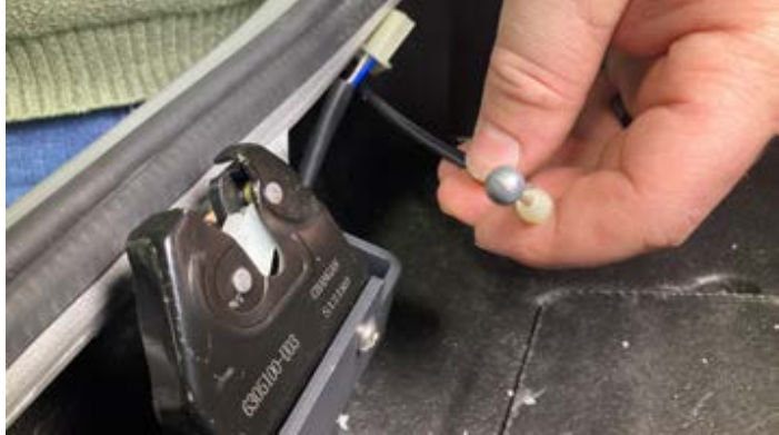
Disconnect the trunk release cable from the trunk latch.
