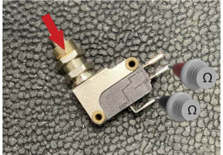
There should be continuity between these terminals when depressed.
