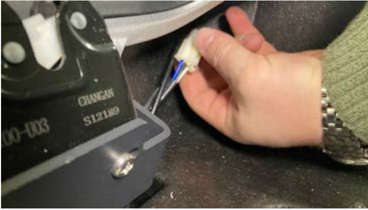
Disconnect the trunk release cable from the trunk latch.
