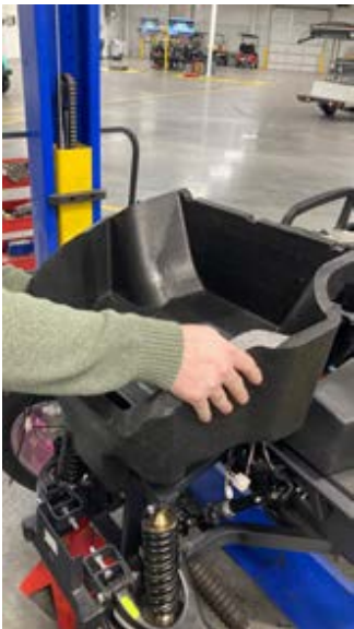
You are ready to pull upward and out, on the front body. You may need an assistant to help with removal.
